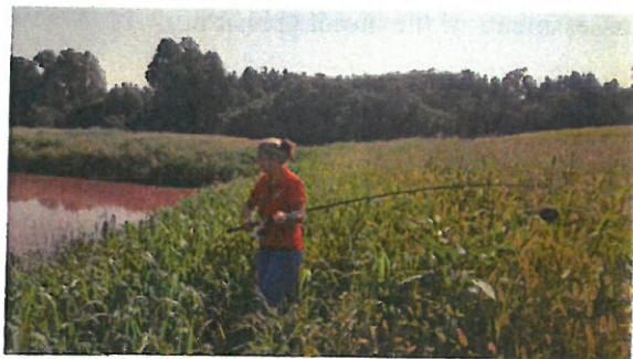
Kim performing a sludge survey with a sonar bobber.
